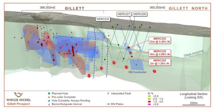
Figure 4 – Oblique 3D view (looking south) showing the basalt footwall, DHEM conductors and additional driling
