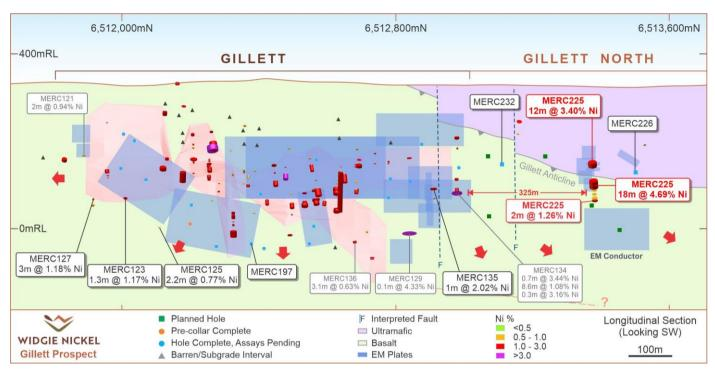
Figure 2 – Oblique long section looking south-west showing Gillett Mineral Resource, MERC225 and DHEM conductors
