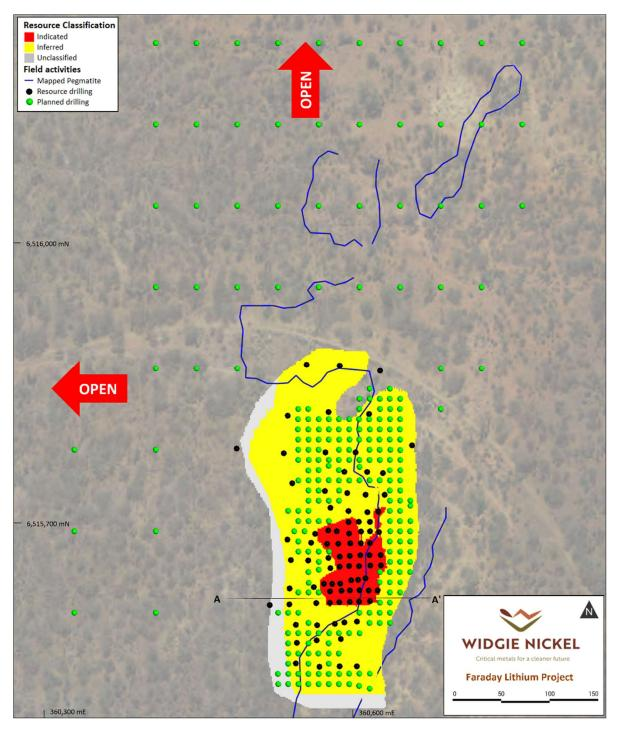
Figure 2 - Faraday mineral resource classification, drilling and pegmatite field mapping
