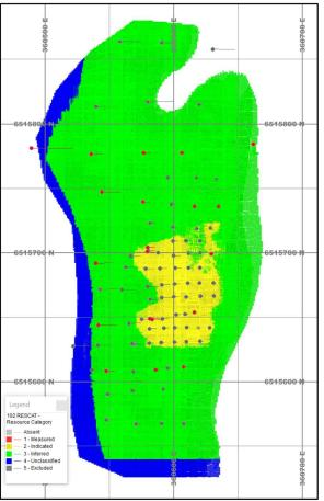
Figure 5 - Plan of drillholes and classification (blue = Unclassified, green = Inferred, yellow = Indicated, grey collars - 2023 and red collars - 2022 drilling)
