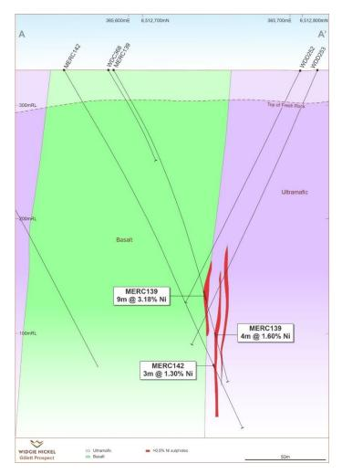
Figure 3 - Gillett cross-section 'B' looking northwest showing MERC139 and MERC142
