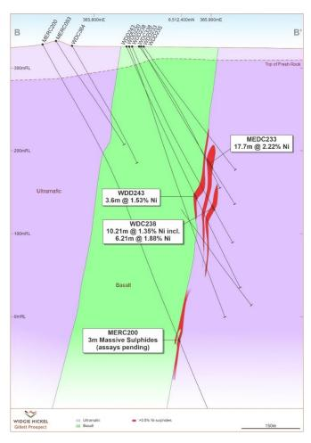
Figure 2 - Gillett cross-section 'A' looking northwest showing MERC200
