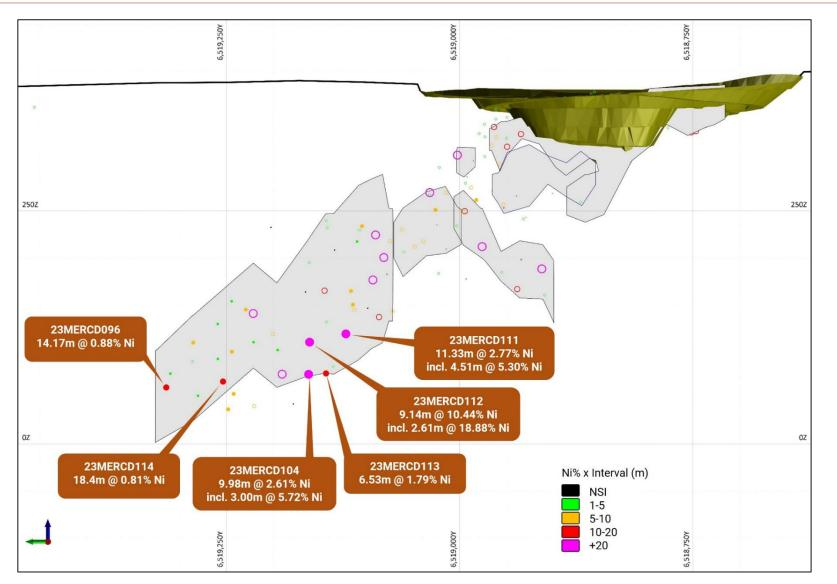
Figure 6: 132N Longsection looking East. Exisitng open pit and 2020 MRE wireframes (grey), nickel % x interval meters solid symbol 2023 drilling, hollow symbol = historic drilling results
