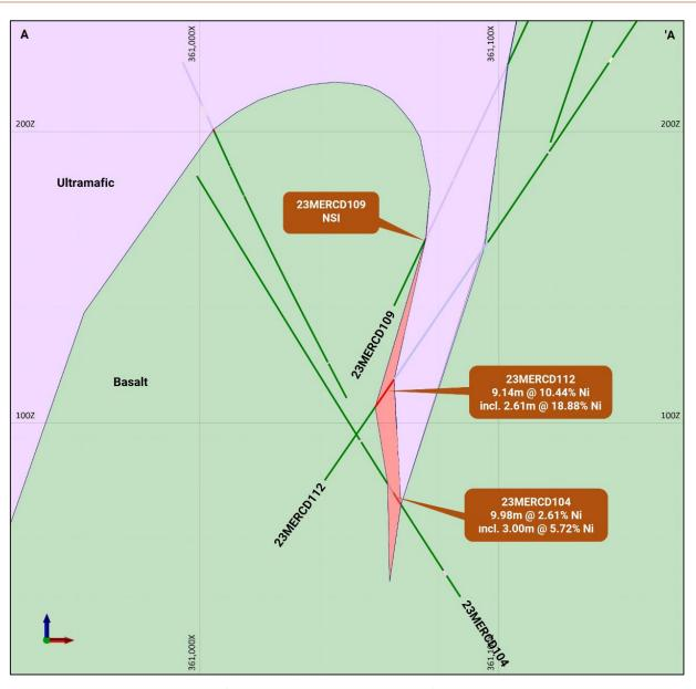
Figure 4: Section A-'A 6519160mN looking north
