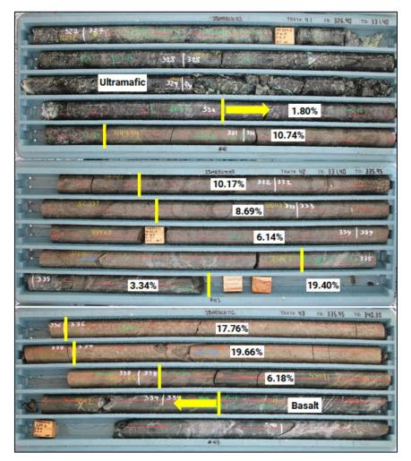
Figure 2: 23MERCD112 displaying individual Ni assay results from disseminated to massive sulphide mineralisation.
