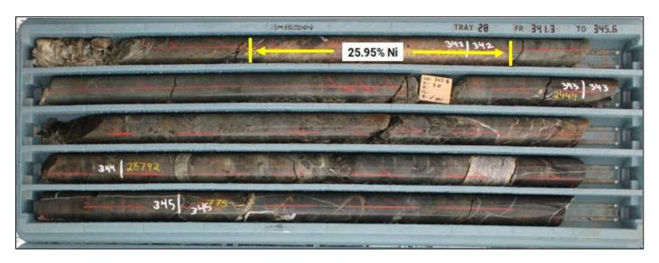
Figure 3: 23MERCD104 displaying massive sulphide mineralisation grading at 25.95% Ni
