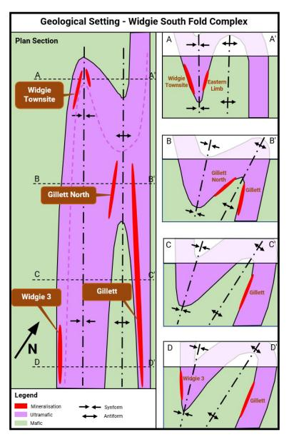
Figure 5: Schematic Geological Setting - Widgie South Fold Complex
