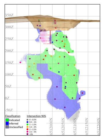
Figure 7: Widgie 3 Classification for the Massive/Matrix Sulphide Mineralisation with Drillhole Intersections – Long Section View looking West
