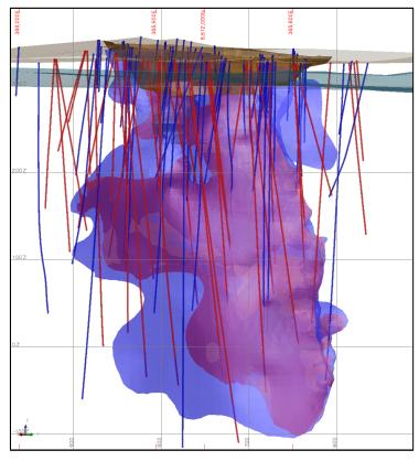
*Figure 6:* Widgie 3 Mineralisation (blue wireframe disseminated, red wireframe massive sulphide domains) and Drilling (red trace 2022/2023) - looking southwest
