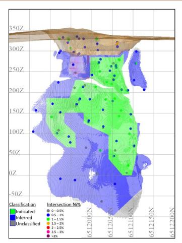
**Figure 8:** Widgie 3 Classification for the Disseminated Sulphide Mineralisation with Drillhole Intersections – Long Section View looking West
