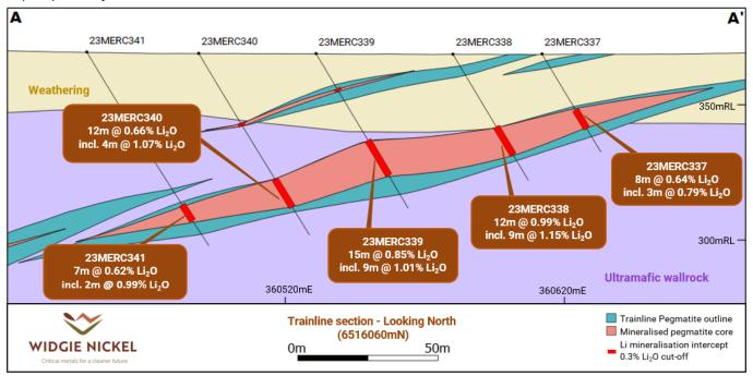
Figure 3 - Cross section 6516060mN, infill drilling at Trainline
