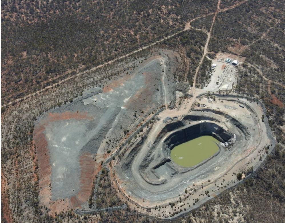
Image 3- 132n Pit with camp and logging facility in background and Armstrong pit water being discharged into open pit in the foreground.
