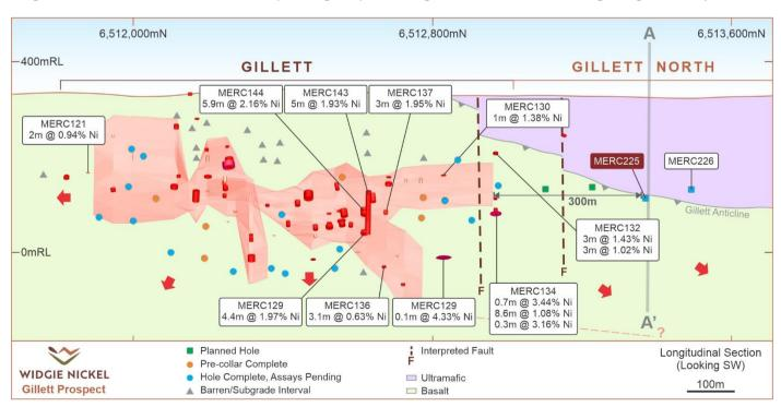
Figure 4 - Gillett long-section (looking SW), showing Gillett North sulphide intervals
