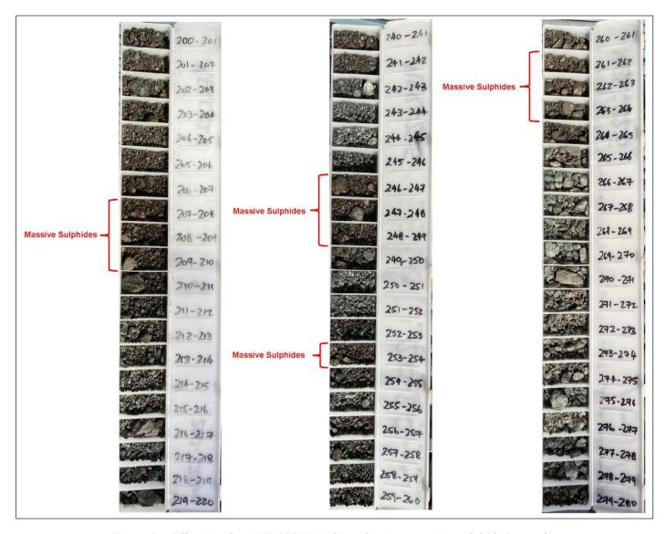
Figure 2 - Gillett North - MERC225 RC chips showing massive sulphide intervals
