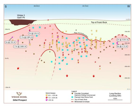
Figure 2: Long section of Gillett looking southwest, showing historical drill intercepts and drillholes planned in the first phase of drilling.
