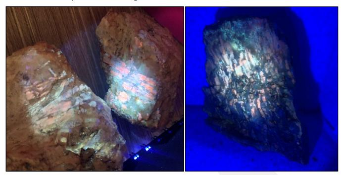
**Figure 1** - Pegmatite samples 24WIN\_SS0043 (left) and 24WIN\_SS0045 (right). Red-orange spodumene under UV light.
