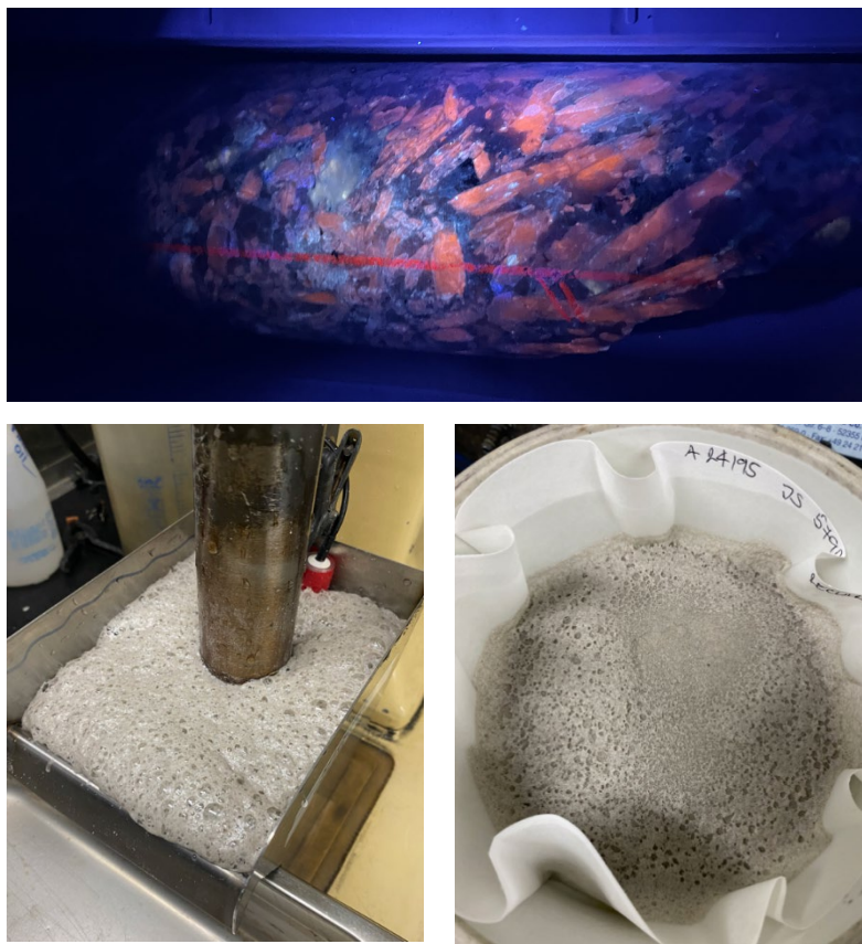
Figure 1 Faraday drill core under UV light, Red/Orange – Spodumene (Lithium bearing mineral LiAlSi 2 O 6 ) Flotation test and Li 2 O concentrate produced
